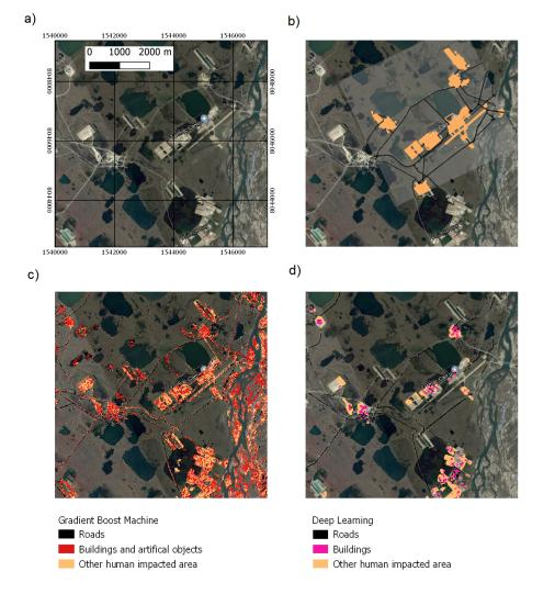
**Figure 10.** Validation data and results for part of the Prudhoe Bay region (WGS 84/UTM zone 5N): (a) Google Hybrid background map, (b) high-resolution validation dataset (area C of the work in [3]), (c) Gradient Boost Machine classification result, and (d) Deep Learning result.
