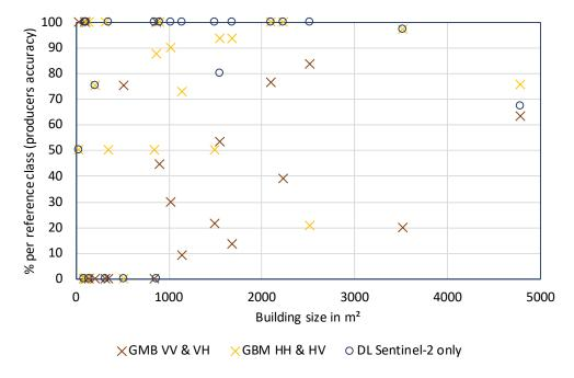
**Figure 13.** Classification performance results with respect to building size in Longyearbyen, Svalbard (validation data source [54]). DL—Deep Learning, GBM—Gradient Boosting Machines, V—vertical polarization, H—horizontal polarization.
