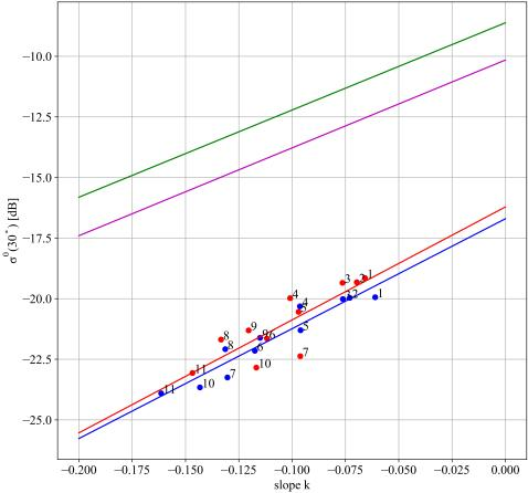
**Figure 5.** Sentinel-1-derived slope values k and  $\sigma^0$  at 30° local incidence angle for most common landcover classes from the work in Virtanen et al. [10] for VH and HV polarization. These values are valid for scenes acquired under frozen conditions in high latitude environments. Previously published HH [53] and VV [51] functions are plotted for comparison.
