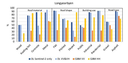
**Figure 11.** Classification performance results for surface types in Longyearbyen, Svalbard (validation data source [54]). DL—Deep Learning, GBM—Gradient Boosting Machines, V—vertical polarization, H—horizontal polarization.
