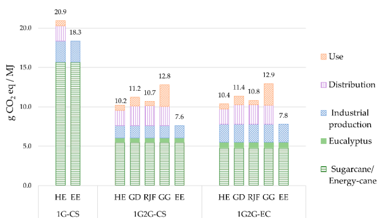
Figure 4. Breakdown of GHG emissions of hydrous ethanol (HE), green diesel (GD), renewable jet fuel (RJF), green gasoline (GG), and electric energy (EE) in the evaluated biorefinery scenarios.
