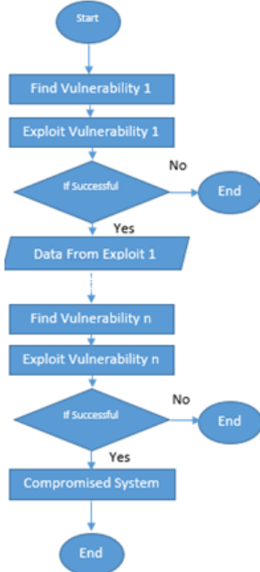
Fig (2) Example of exploit chain with multiple vulnerability
