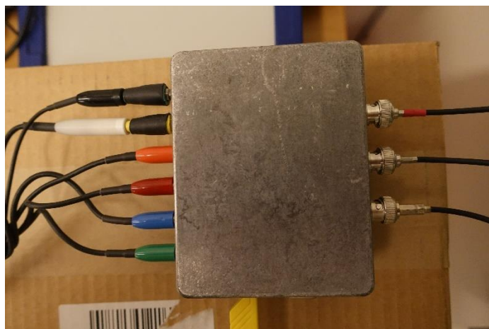
Figure 15: Protected connection box between original cables (left) and coaxial cables to the electrochemical cell (right).
