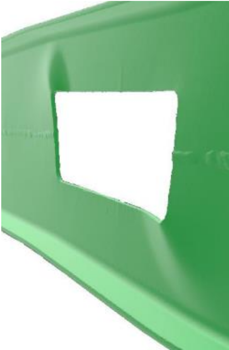
Figure 12: Post-test deformations of Specimen B [7].
