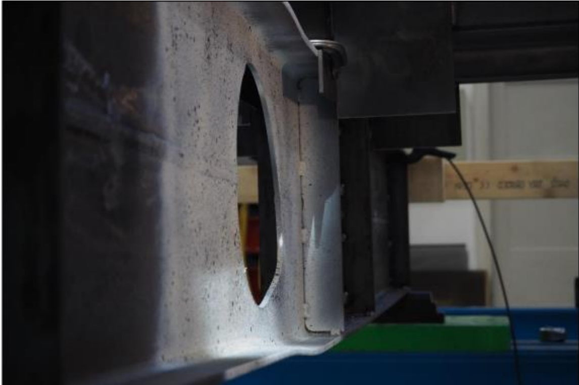
Figure 17: Post-test deformations of Specimen D [6].
