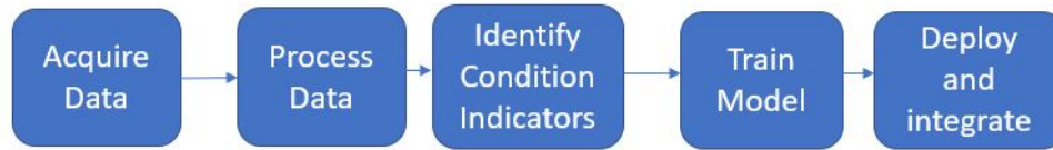
Figure 4.1: Steps to design predictive maintenance algorithm Failure prediction adapted from [Li, 2018]
