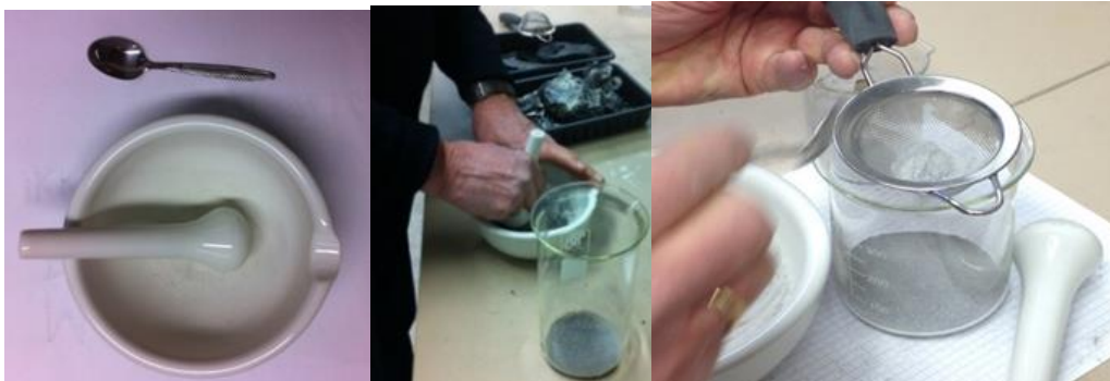
Figure 3. The forehead bones ground in a mortar and then sieved. Sieve mesh aperture: 1 \times 1 mm.
