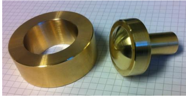
Figure 7. The cupel tool, ring (left) and the 'monk' (right).
