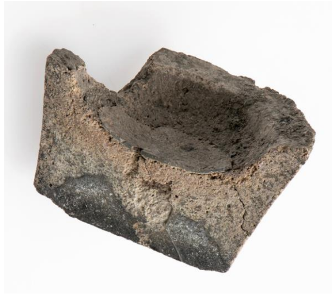
Figure 14. A cross-section of the excavated cupel N124860. The upper, outer rim diameter is 35 mm and the height 23 mm. Note the fine-grained surface layer (i.e. the facing) at the bottom of the bowl. The two dark areas at the bottom of the cupel show where lead oxide has filled the cavities between the bone-ash particles, as well as the interior of the particles (see Figure 16). Photo: Åge Hojem, NTNU University Museum.
