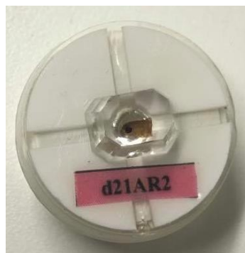
Figure A2. Lumpfish embedded in resin on a block holder. A 21 dph Art-larva embedded in resin. The larva has been cut behind the anus in the transversal plane prior to embedment.
