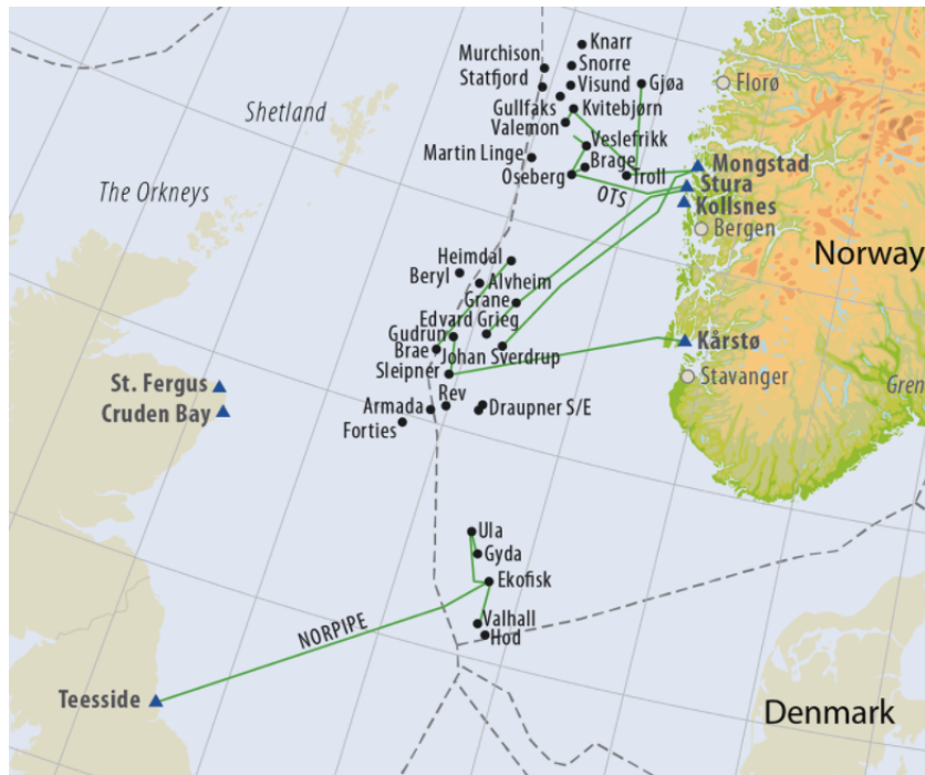
Figure 6: Representation of the pipeline system for oil and gas condensate. Figure derived from Norwegian Petroleum (Norwegian Petroleum, 2021d).
