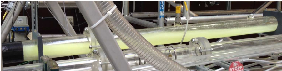
Figure 7.12: Flow pattern after expansion. Water flow rate 5.8 kg/s, air flow rate 5 g/s. 2.7° inclination.
