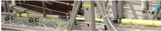
Figure 4.7: Shut-in valve mock-up with green dyed water.
