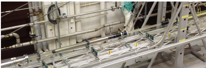
Figure 4.6: Shut-in valve mock-up in multiphase laboratory.
