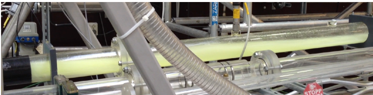
Figure 17: Flow pattern after expansion. Water flow rate 5.8 kg/s, air flow rate 5 g/s. 2.7 deg. inclination.
