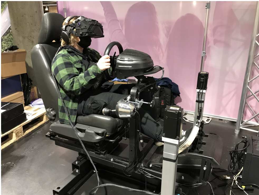
Figure 3.3: The VR simulator at Way, which was used to conduct the tests. The test subject was able to drive independently through the night driving course.
