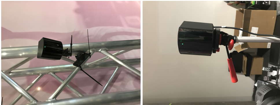
Figure 3.8: Valve tracking stations to improve the headset tracking accuracy and stability.
