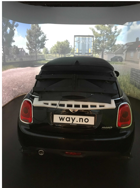
Figure 2.10: A monitor is mounted at the back of the car's rear window in Way's CAVE simulators.
