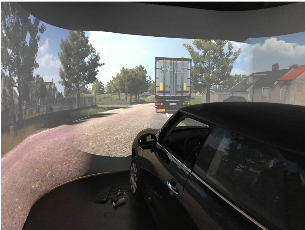
Figure 2.12: A CAVE simulator at Way that is used to conduct driving training in an alternative way.
