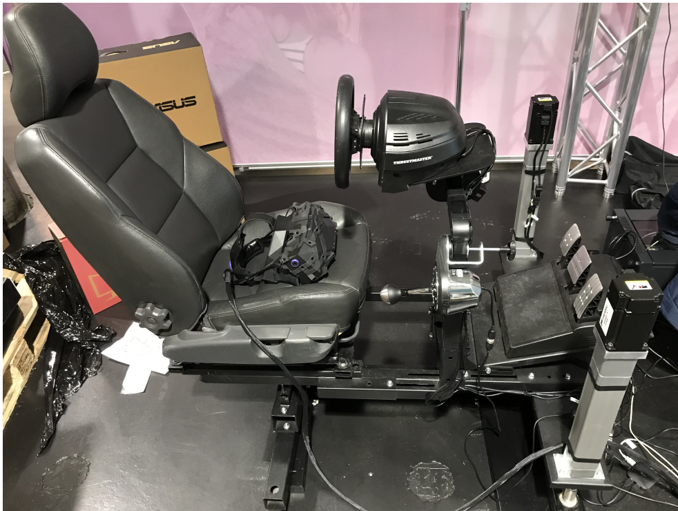
Figure 2.4: The VR simulator at Way, which was used to conduct the test in this thesis.
