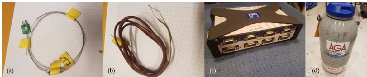
Figure 7. (a) Thermocouple type K, (b) thermocouple type T, (c) QuantumX DAQ module, and (d) cryogenic capsule.
