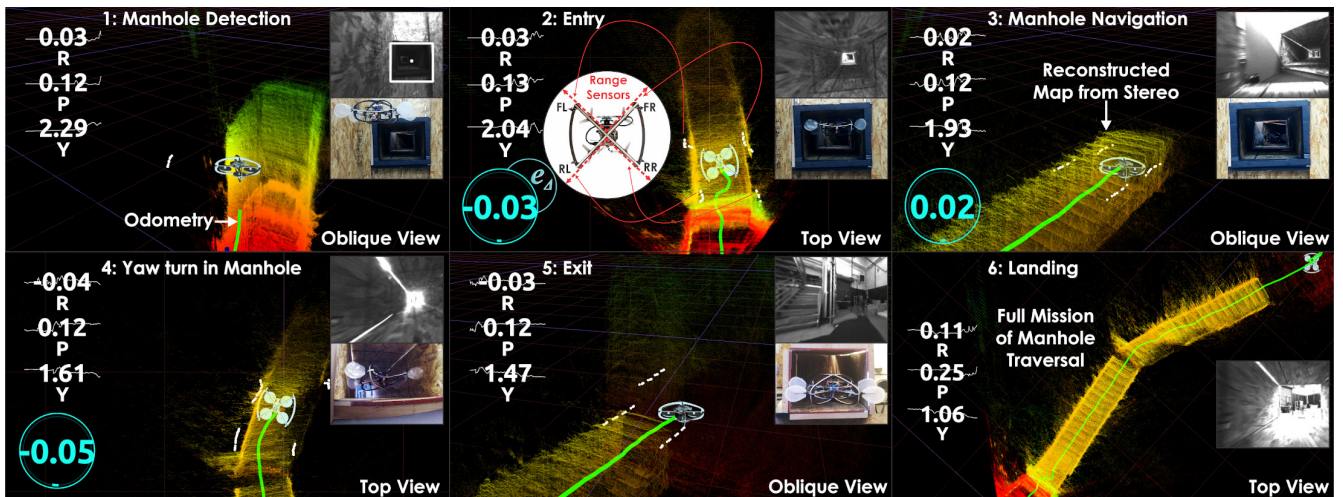
Fig. 5. Instances of an experiment of an autonomous collision-tolerant navigation of a non-straight manhole tube (width \times height = 0.5 \times 0.4 m) with a total length of 5.2m. RMF resiliently traverses this tight environment by exploiting its compliant flaps which ensure smooth contact with the environment. After a successful detection and localization of the manhole (1), the robot enters the manhole (2) and subsequently “locks” a forward pitch (P) command (3). It minimizes the sum of the left and right diagonals (bottom left turquoise circle) to keep the yaw aligned with the tube (4). Using its TOF sensors, the system is then able to detect the exit of the tube (5) and safely land outside (6). Instances of the mission and of the onboard camera are also presented.
