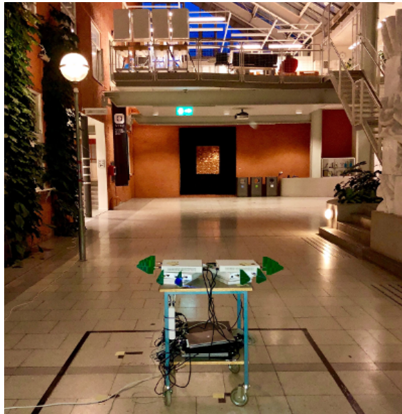
Figure 4.3: Positioning of the base station on the balcony and the user equipment cart. The antennas are pointing away from the balcony to illuminate non-line of sight links. Five physical locations in the black square were measured for each frequency band.
