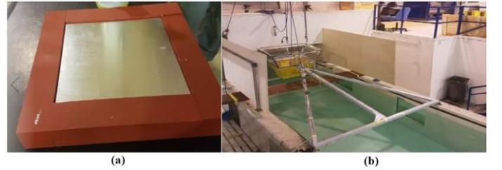
Fig. 2. (a) Test specimen of aluminum plates; (b) setup of the drop test, from Abrahamsen et al. (2020).
