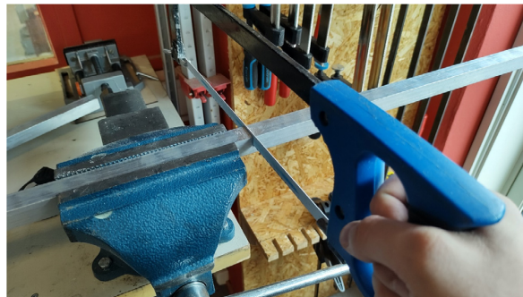
Fig. 15. Saw the aluminum profile before drilling holes in it.
