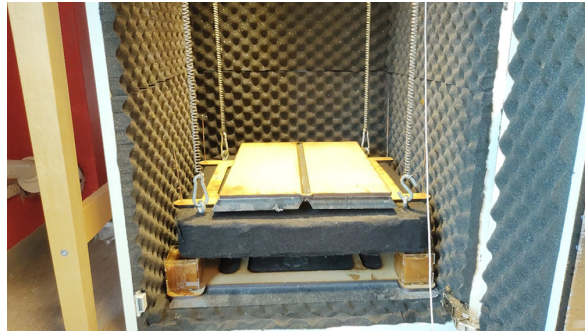
Fig. 34. Table in its final operating height with steel plates as weights.
