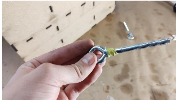
Fig. 21. Gasket made of vacuum bagging sealing tape.
