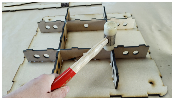
Fig. 18. Use a hammer to force the inner structure together with the top plate.
