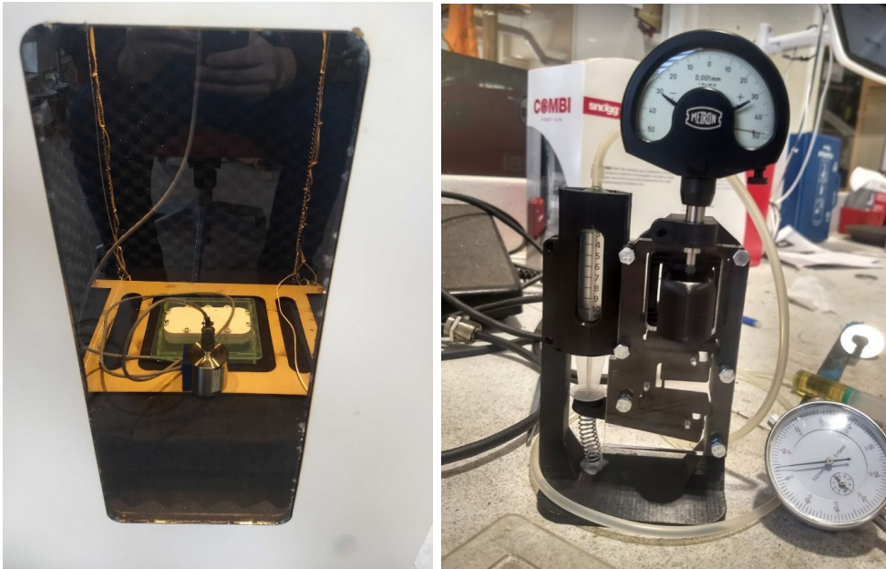
Figure 4 - To the right, chamber with a table isolated against external mechanical vibrations. To the left, a compliant mechanism driven by pistons for small compression tests of sensor materials
