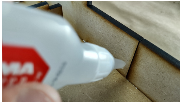
Fig. 20. Add CA glue to fix tricky alignments quickly.
