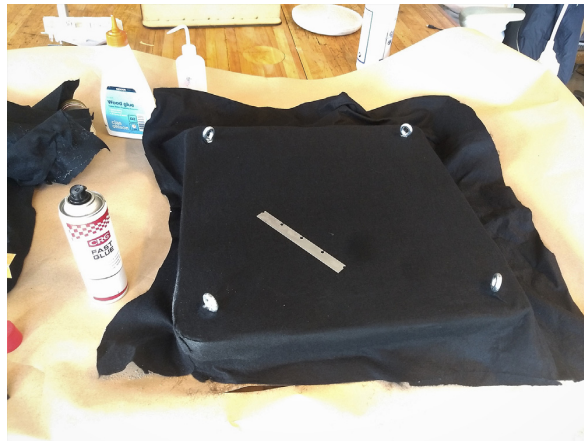
Fig. 24. Felt added to the top of the table.
