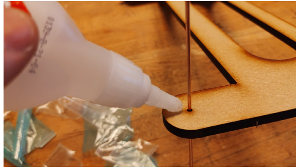
Fig. 32. Insert damper rods into plate and apply CA glue.
