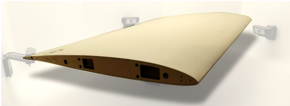
Figure 15 - Wing for test. Hole pattern for mounting can be seen on the side.
