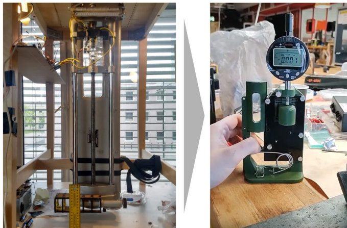
Figure 22 - To the left, a tensiometer stretch bench which is driven by a worm gear. To the right is a 3d-printed compliant mechanism alternative.
