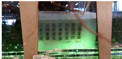
Fig. 3. Wing with integrated sensors in water tunnel.
