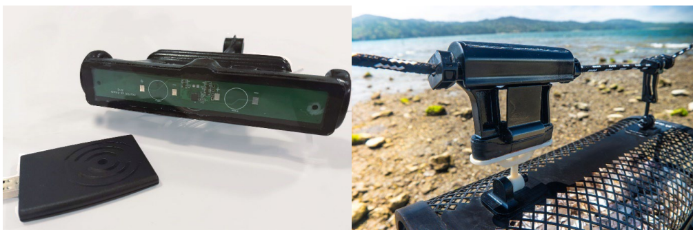
Figure 2 - The connecting hooks of the oyster farming system contains load cells and passive UHF RFID modules. Right photo by: Marius Auflem (2019) reproduced with permission.
