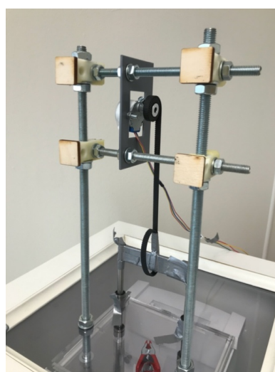
(II): Closeup of the upper part of the lifting mechanism.
