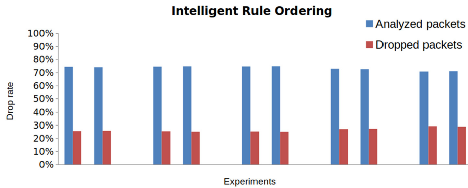
Fig. 6. Results of five packet drop rate experiments using two Snort sensors with intelligent rule ordering.
