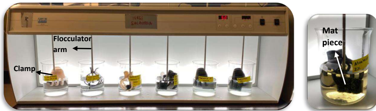
Figure 6: Mat piece ca 5x2.5 cm dipped into enzymatic solutions attached with a clamp to the flocculator arm.
