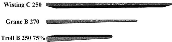
FIG. 3. Accumulation of the 10l oil slick in front of ice floe for (a) Wisting central 200 °C, (b) Grane 270 °C, and (c) Troll B 250 °C 75%emuls. at a current velocity of 20 \frac{cm}{s} (for simplicity, only the oil slick is illustrated).
