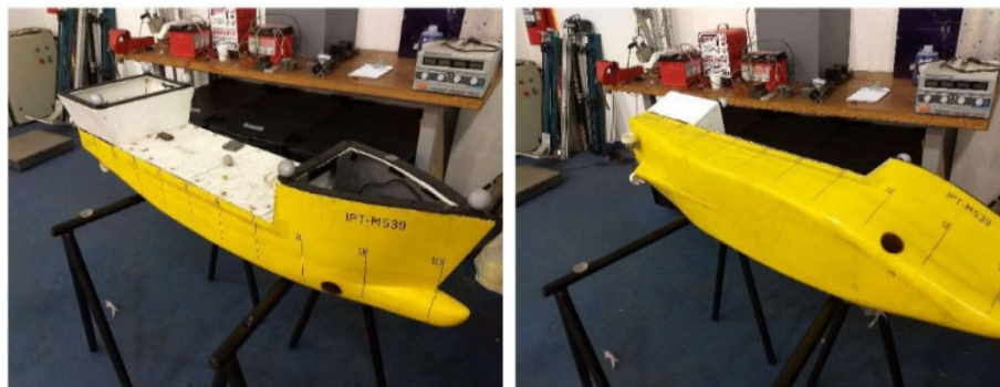
Fig. 4. Scale model PSV used during the experiments [30]. Six reflective, spherical markers for motion tracking were attached to the model.
