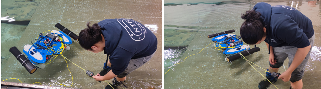
FIGURE 3.2: Measure the thruster force of Double Blueyes Robot
