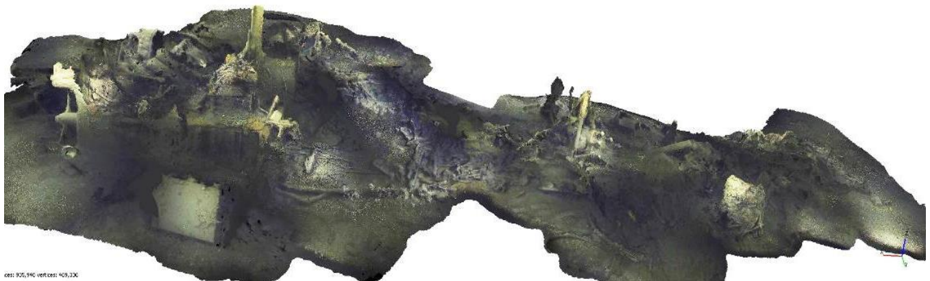
Fig. 7. Photorealistic 3D model of the wreck site, created by fusing imagery data of two surveying periods (2019, 2021).
