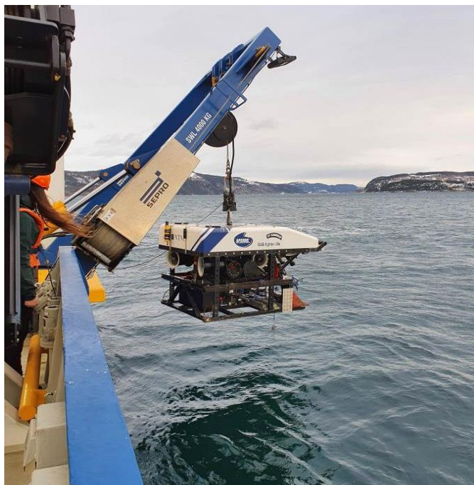
Fig. 2. Setting up the multi-cam system. An omnidirectional system of six GoPro cameras and an individual GoPro are mounted in the front of the ROV, facing different perspectives of the seabed and the wreck. The chessboard pattern was used for the intrinsic and extrinsic calibration of each camera.
