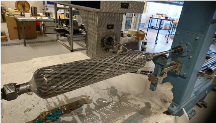
Fig. 3. Winding of the first axial layer of the pressure vessel. Rings for testing were cut from the cylindrical part.
