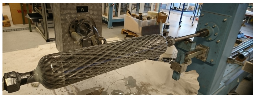
Figure 2. Winding of the first axial layer of the pressure vessel.
