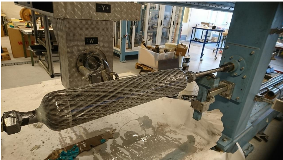
Figure 6 The filament winding machine at NTNU winding a low angle glass fiber reinforced polymer layer. The rx axis is labelled "W" on the impregnation chamber.
