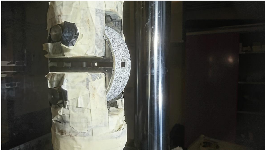
Figure 11 The split disk test setup used in this thesis. White tape is used on the steel tension arms to hinder reflections of light for DIC cameras.
