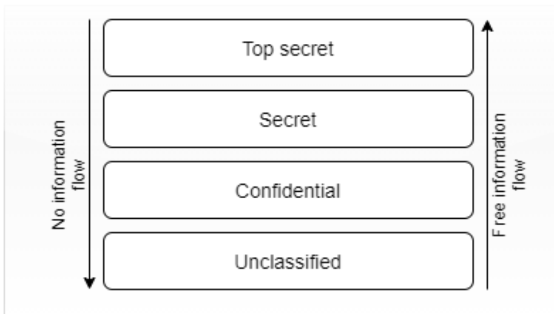
Figure 6.2: Multilevel security in which sensitive information is protected by classifications and clearances
