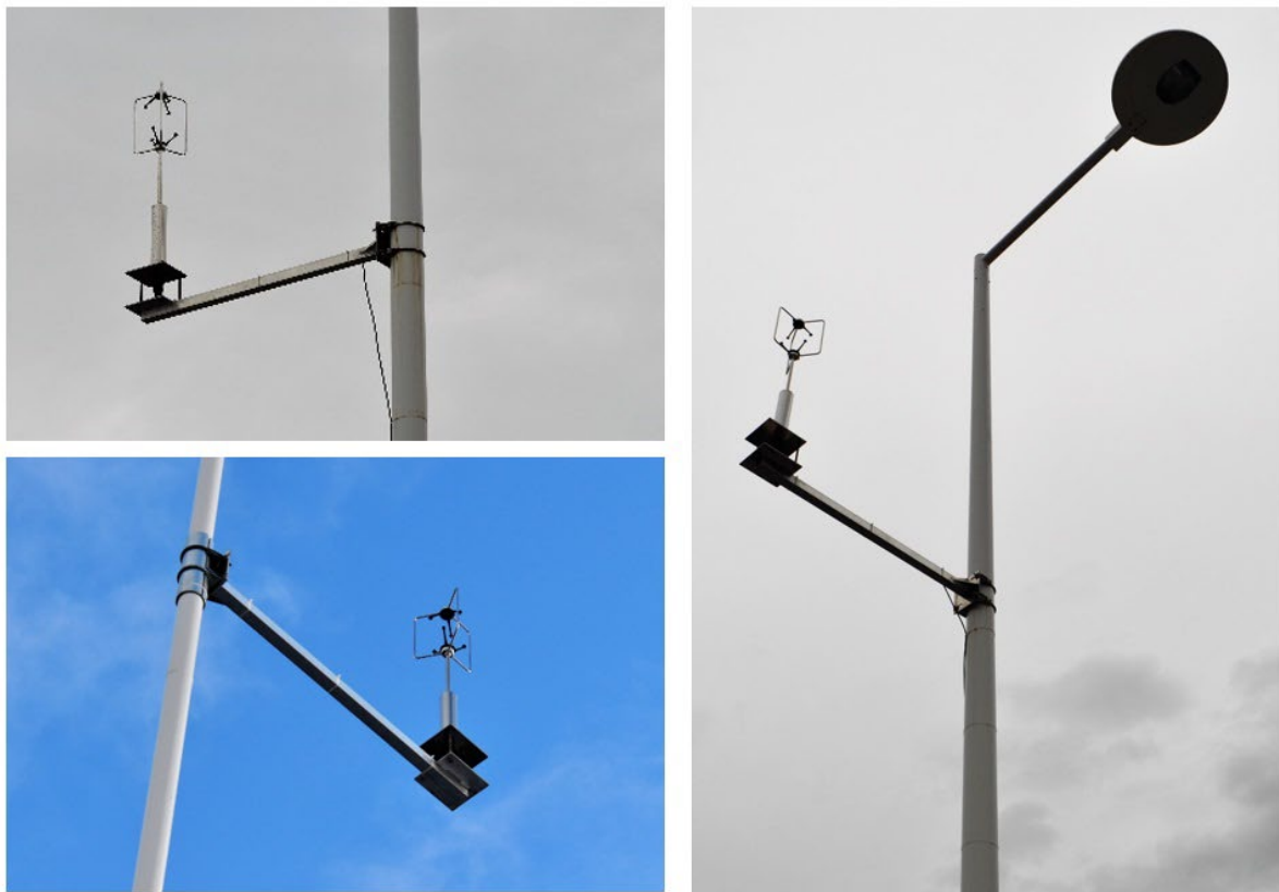
Figure 7 Anemometers on the bridge. On the right side, anemometer A6 is shown, which is attached to a light pole on the West side.
