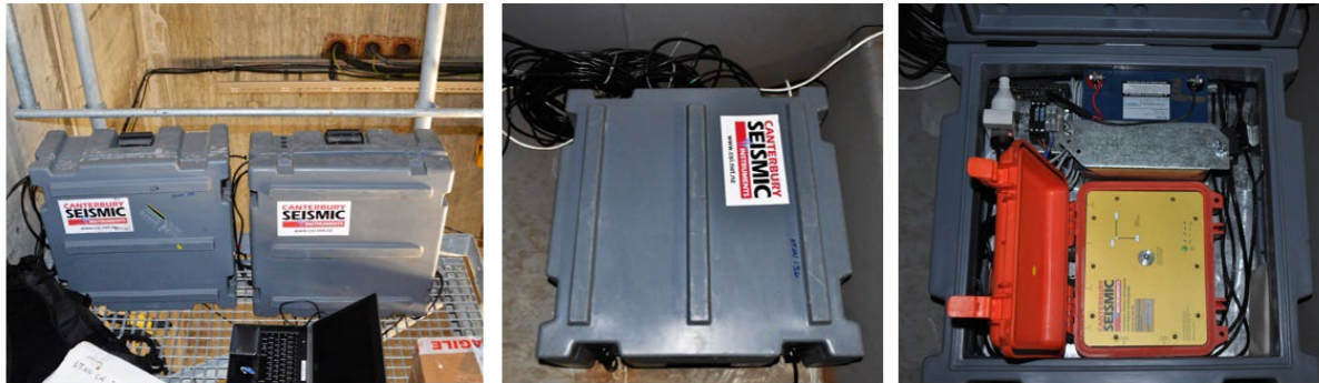
Figure 8 Datalogger units. Inside each gray box, there is a datalogger unit, a battery and a charger. The measuring sensors, GPS sensors and Wi-Fi antennas are connected to the logger by wire.
