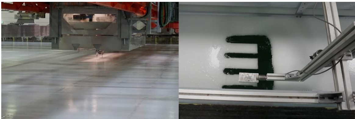
Figure 3. Testing level ice flexural strength
