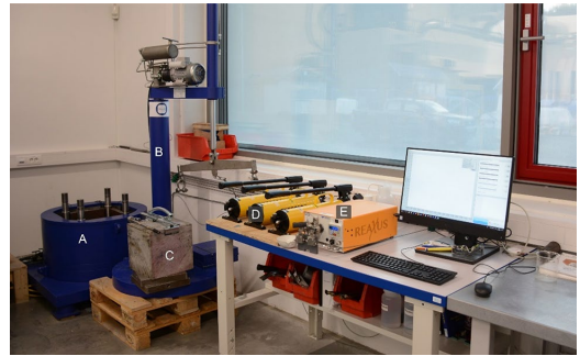
Fig. 3 Overview of the test rig. From left to right is a the test frame, b the integrated hydraulic crane, c one of the granite specimens resting on the top lid, d three hand pumps used for pressurizing the hydraulic pistons, e the high-pressure pump used to pressurize the test section, and the desktop computer where tests are controlled and monitored
