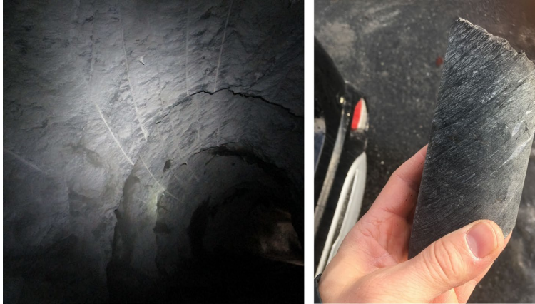
Fig. 4: Examples of phyllite encountered at the lower parts of the pressure tunnel. To the left is the excellent tunnel contour observed at the test location, and to the right a core specimen of the rock. Note the distinct foliation and thin white bands of quartz, characteristic for the rock type
