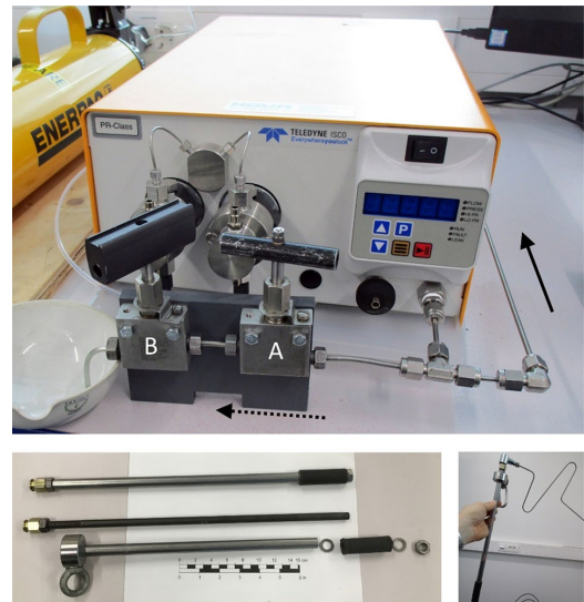
Fig. 6 Injection pump and packer assembly. Top: pump with valve configuration enabling flow-back. Unbroken arrow indicates flow direction during injection, dotted arrow shows direction during flow-back and venting. The lower left picture shows the injection packer with scale indicated. Note, the in-house modification of the upper part of the packer rod, incorporating an eye bolt for secure anchoring of the packer during testing. The expansion loop in the steel pipe is shown in the lower right photo
