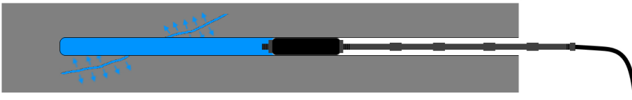
Figure 3 Mechanical packers used to isolate the test section
