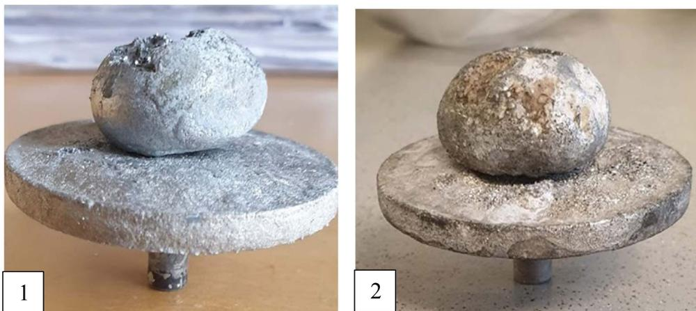
Figure 10. Deposits using NaF-AlF<sub>3</sub> cryolite, CR = 2.2, CCD = 0.9 A cm<sup>-2</sup>, t = 4 h, (1) T = 980 °C, 2 wt.% Al<sub>2</sub>O<sub>3</sub> at 1 wt.% Si, (2) T = 970 °C at 1 wt.% Si.
