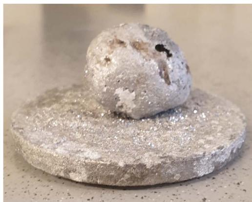
**Figure 8.** Deposit using NaF-AlF<sub>3</sub> cryolite with no alumina feeding at 3 wt.% Si, CR = 2.2, CCD = 0.9 A cm<sup>-2</sup>, t = 4 h, and at 980 °C.
