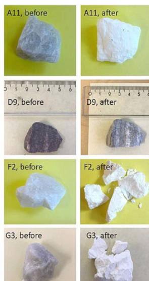
Figure 7: Sample A11 heated to 1700 °C and held for 60 minutes, sample D heated to 1600 °C and held for 45 minutes, sample F heated to 1600 °C and held for 120 minutes, sample G3 heated to 1700 °C with no holding time. Pictures of the sample before and after heating of the sample can be seen. All the samples are around 10 g and 2-3cm large.
