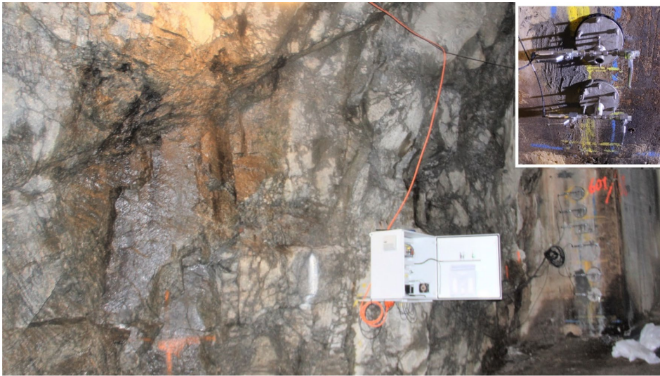
Fig. 10 Location of datalogger in the construction adit. Arrangement of pressure transducers and deaeration valve is shown in top right corner
