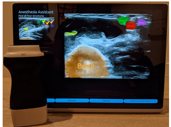
Fig. 5. Real-time prototype consisting of a FAST application, a Surface Book laptop and a Clarius L15 HD scanner.
