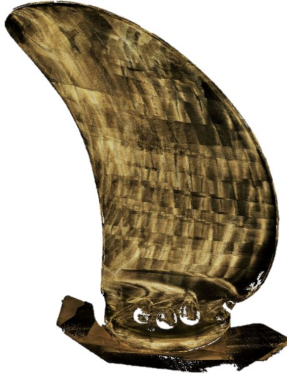
Fig. 8: 3D inspection results using the proposed approach with an industrial robot and a high-accuracy RGBD-camera.
