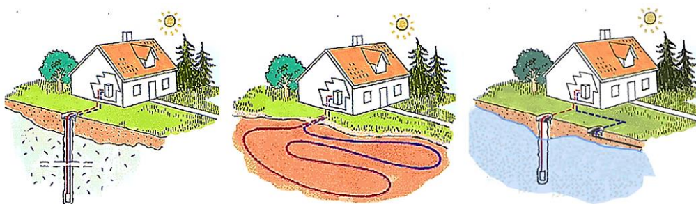
Figure 1-2 Common types of ground coupled heat pump systems. ( left ) Energy wells in bedrock ( in-direct closed loop system ). ( middle ) Horizontal pipes in dug ditches. ( right ) Groundwater systems that pump groundwater from aquifers ( direct system ). Modified after Normann Etek AS (source unknown).
