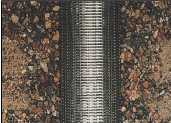
Figure 2-2 A typical con-slot well screen utilized in Norwegian groundwater wells. The well conditioning removes the fine particles in the vicinity of the well screen and the remaining soil material function as a naturally developed filter (Driscoll, 1986).
