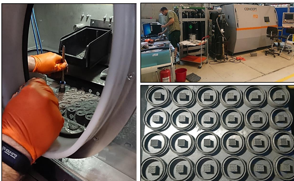
Figure 3-6 Additive manufacturing facilities at the NTNU AM laboratory in Trondheim and at SINTEF Manufacturing AS. (Left) Cleaning of the samples after fabrication. Health and safety measures are important because the microscopic Marlok C1650 powder particles are very fine. (Top Right) Vegard Brøtan is preparing the Concept Laser M2 PBF-LB machine with the four CAD models. The building chamber is within the grey machine to the right. (Bottom right) A failed test specimen of Samples A-D shows the first 1 cm of fabrication. The machine can fabricate all 24 samples simultaneously. This required one full week of continuous fabrication.
