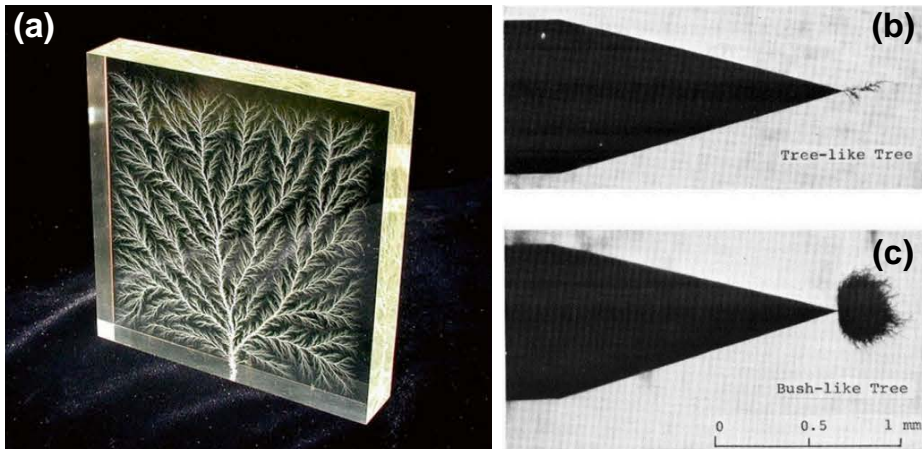
Figure 2.16. (a) The profile of electrical trees in poly(methyl methacrylate), and the formation of (b) linear (tree-like) trees with few branches, and (c) bush-like trees with multiple branches close to the initiation point, in polyethylene. Both images are reprinted with permission from Springer Nature Customer Service Centre GmbH: Springer Nature, Polymer Nanocomposites Electrical and Thermal Properties by Xingyi Huang and Chunyi Zhi, 2016.
