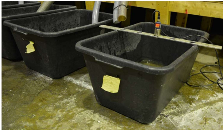
Figure A.1: Measuring the water height in the bucket by pouring 1L of water into it.
