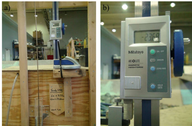
Figure B.1: Setting up the water level of the reservoir using point gauge on the right and piezometer on the left.
