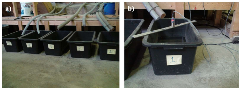
Figure 14: a) Five buckets for collecting the overtopping volume; and b) Ultrasonic sensor for measuring overtopping volume (Photo: Netsanet Nigatu, NTNU).
