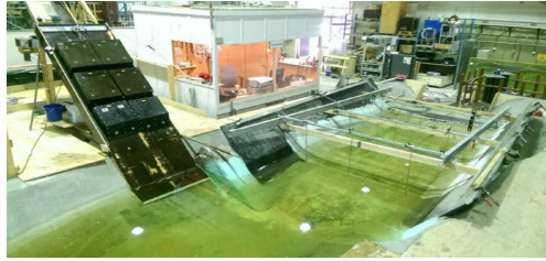
Figure 6. Model setup for the landslide and reservoir model, Photo: Kiflom Belete
