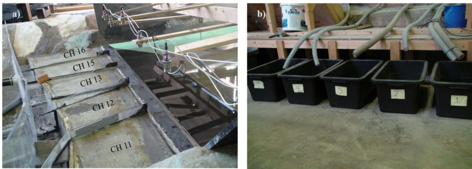
Figure 12: Picture of dam crest sections, CH 11 through CH 16 on the left and five buckets collecting overtopping water at each dam section on the right.
