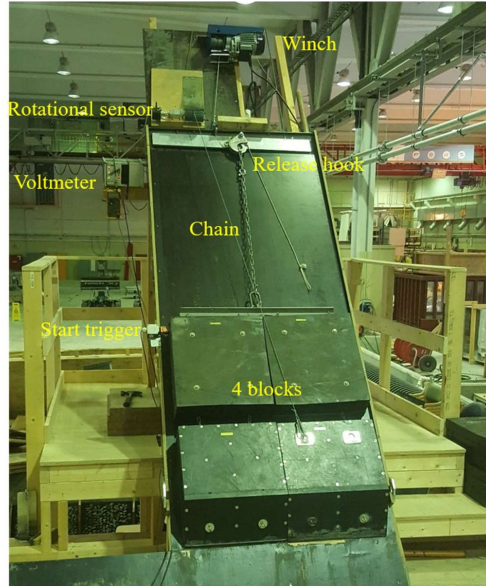
Figure 9: The slide ramp where 4B are placed to slide into the reservoir.
