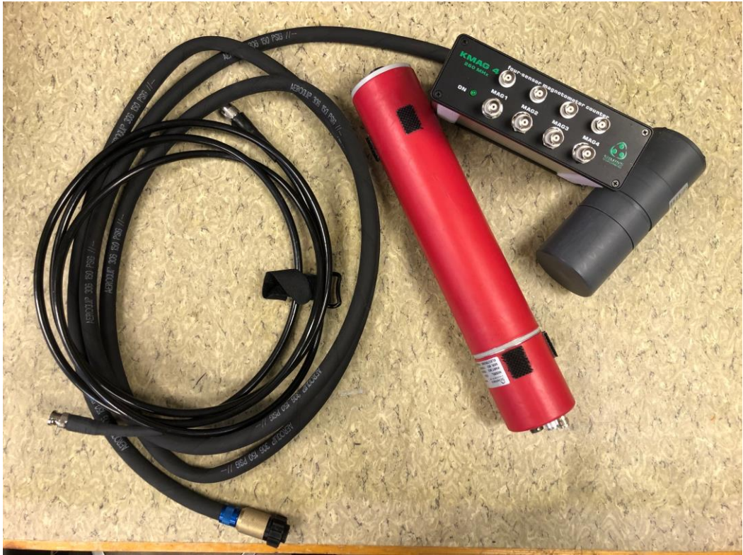
Figure 2.10 Example of Caesium vapor magnetometer used for NGU helicopter survey. The black cylinder contains the sensor, the red cylinder is the amplifier and the black box labelled KMAG 4 is the magnetometer counter.
