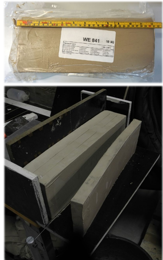
Figure 4.5. Above: Wrapped pottery clay block. Below: cut block.
