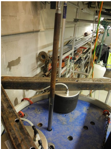
Figure 4.43. Penetrometer fixed to rod, placed above sub-sample 2a.
