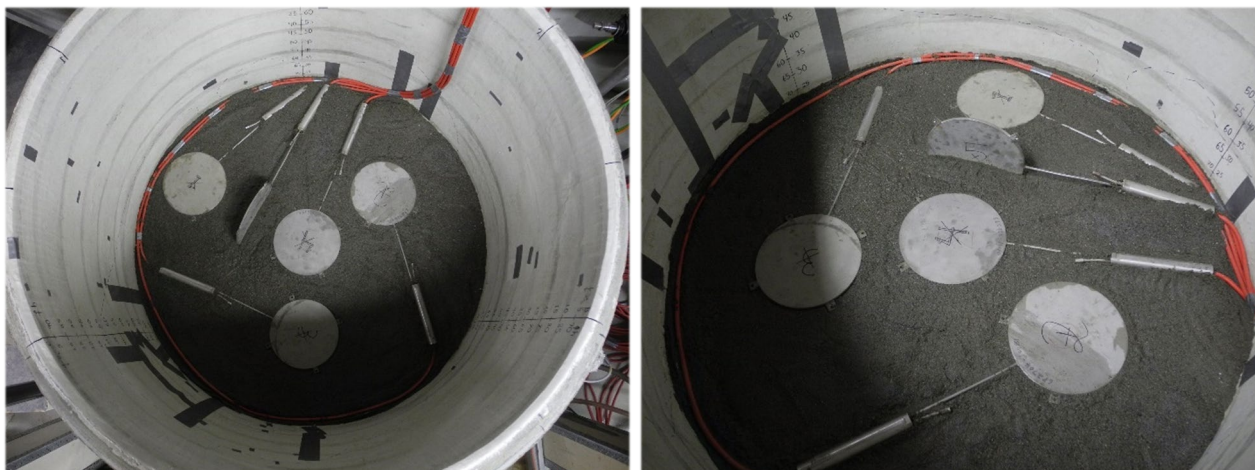
Figure 4.24. The pressure cell set-up in experiment 2 and 3, from different angles.
