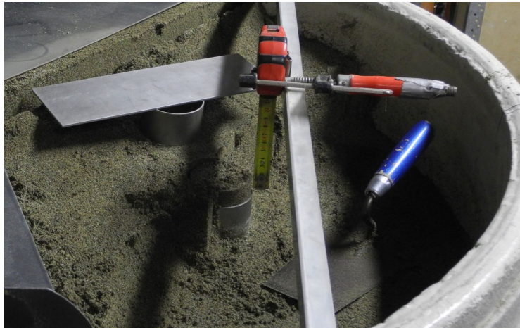
Figure 4.45. Picture from during a density test.
