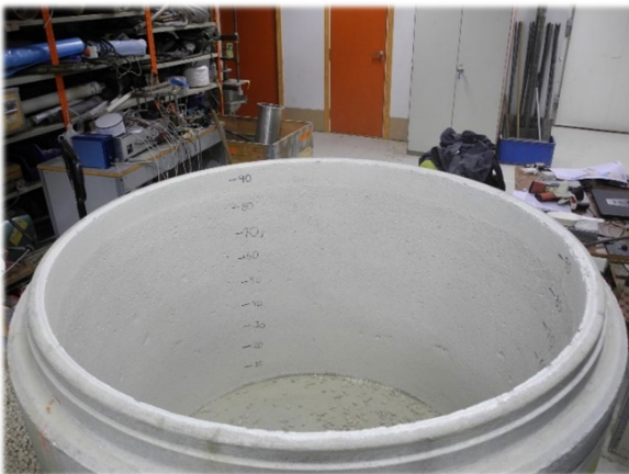
Figure 4.2. Chamber base, with some guiding height lines.
