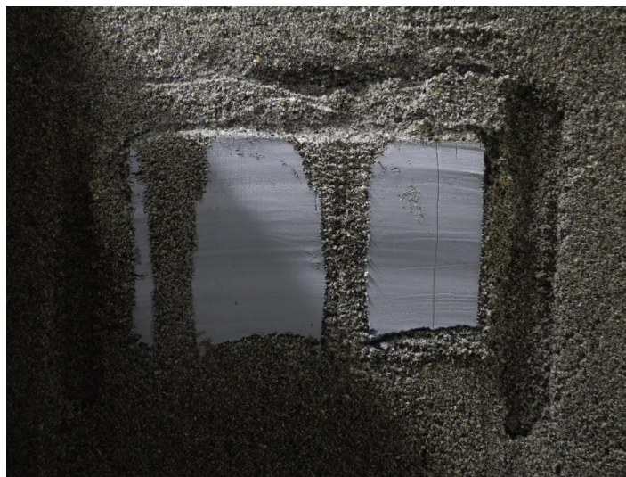
Figure 6.6. Cylinder at the lowest level in sector a. The penetration of sounding 3a was completely confined by clay. The unit in section a was shifted relatively away from the original chamber wall. The disc at top remained fixed due to the artificial load framework fixed position.
