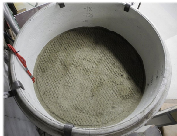
Figure 4.13. 1 st phase, newly rained sand.
