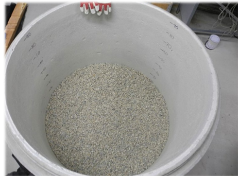
Figure 4.9. The first 10 cm of the chamber was filled with gravel.
