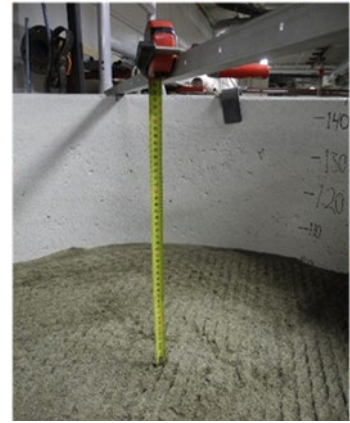
Figure 4.20. Height measurement device. Measurements were made after every phase.
