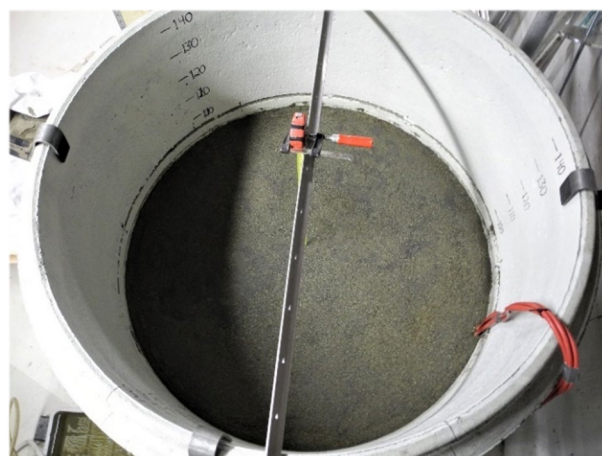
Figure 4.15. After 4 th phase, water discharge, followed by vibration.
