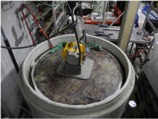
Figure 4.16. 4 th phase, plate vibrator on wooden plate.
