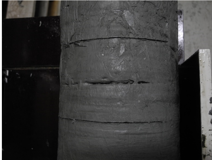
Figure 6.12. Most likely an intermediate siltier layer in a mini-block consisting mainly of quick clay.
