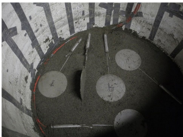
Figure 4.25. Slightly inclined pressure cell. It appears more inclined in the picture due to camera angle.
