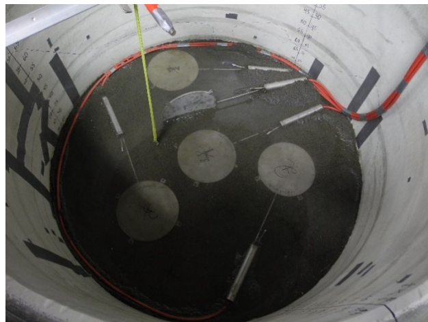
Figure 4.26. Zero-calibration procedure, with cells submerged under a 5 mm water film.
