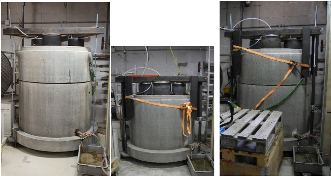
Figure 4.39. Loading framework, initial (left), redesign with chamber base (middle) and extension (right).
