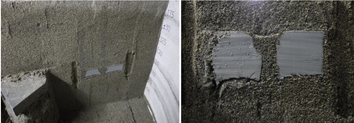
Figure 6.7. Left: Upper clay layer of sector a, sounding 3a went through the very perimeter. Right: Middle clay layer of sector a, sounding 3a went somewhat inside the perimeter.
