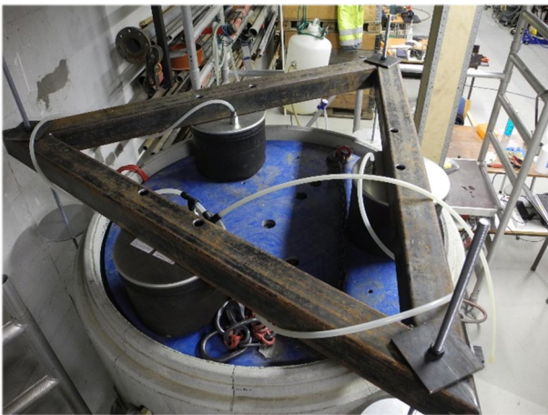
Figure 4.40. The framework with bellows and rods.
