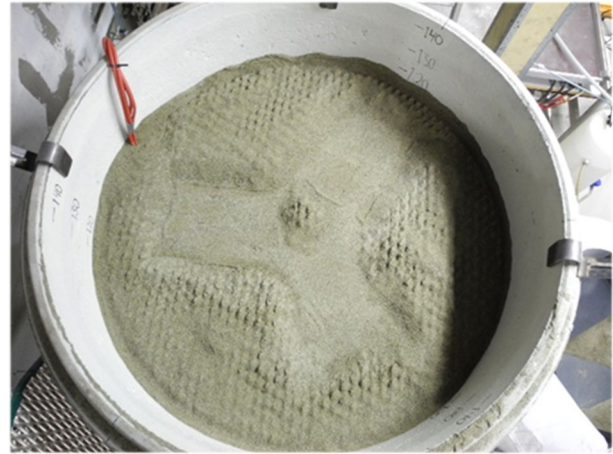
Figure 4.17. Sand layer thicknesses adjusted the clay units' heights.
