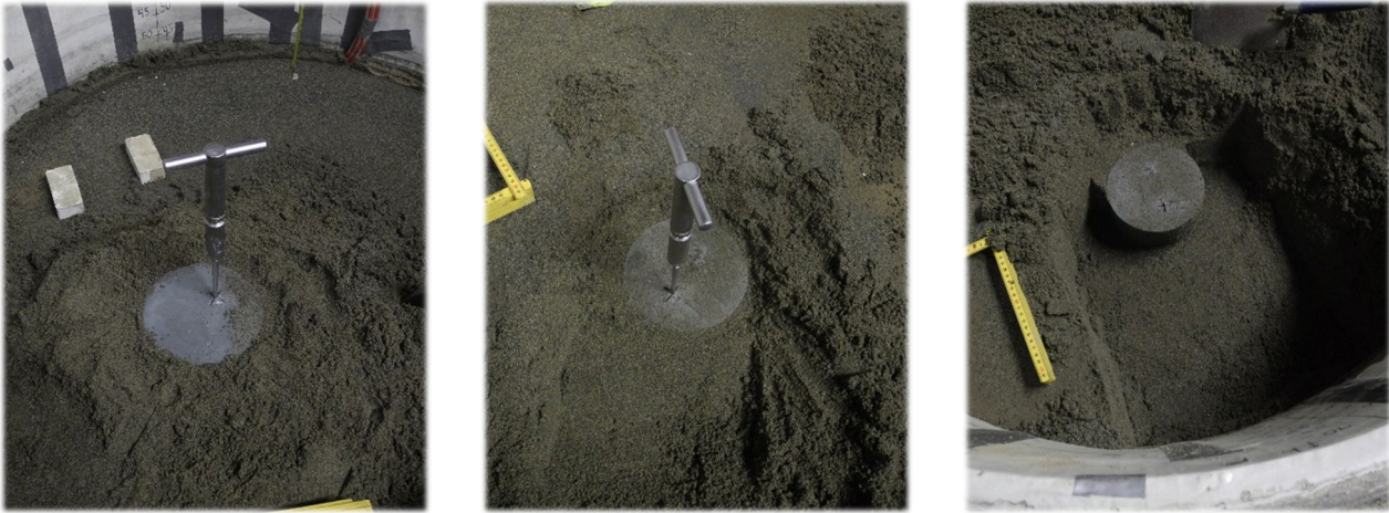
Figure 4.6. Pocket vane test prior to (left), and after (middle), build-in. Excavated intact specimen (right).
