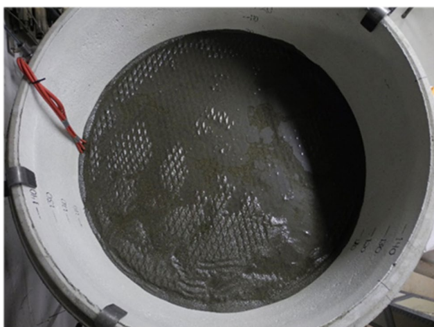
Figure 4.14. 2 nd phase, fully saturated sample, excess water on top.
