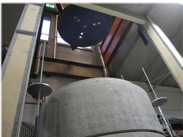
Figure 4.37. Metal disc and loading framework lowered unto the sample.
