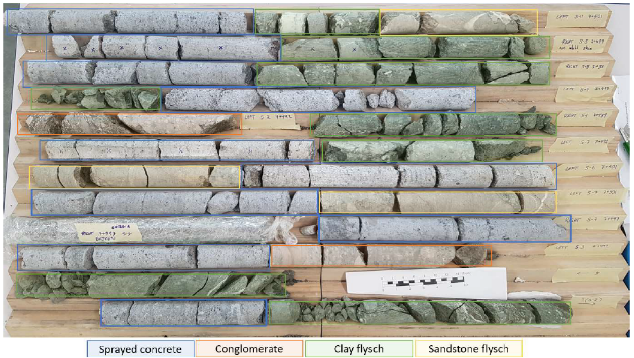
Figure 8.1: Rock samples extracted from Moglice headrace tunnel from chainage 7+492 to 7+501 (Photo by Runa B. Frengen (Frenge, 2020))
