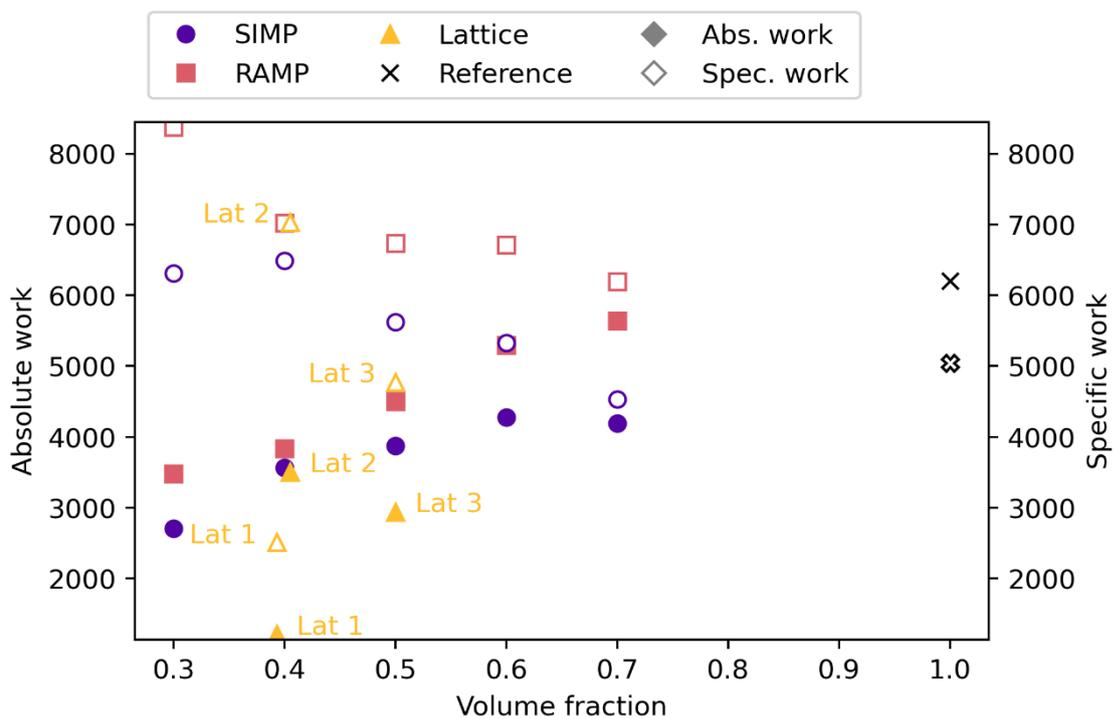
Figure 19: Absolute and specific work of fracture  $U$ .
