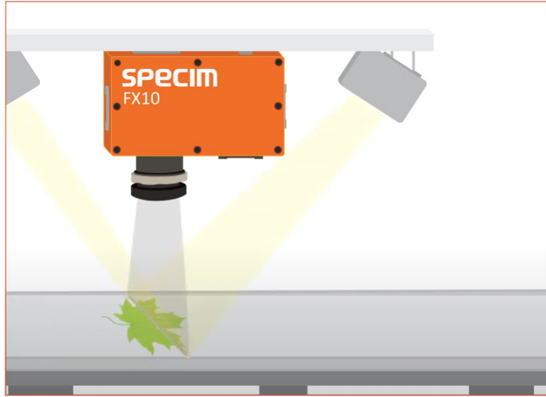
FIGURE 5.8: Illustration showing the push-broom technique. Courtesy of Specim (n.d.[b]).
