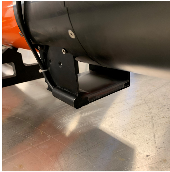
FIGURE 3.6: SilCam mounted on LAUV Road.
