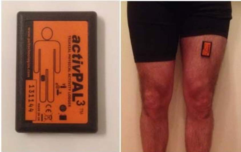
Figure 1. The activPAL activity monitor (left) and a participant with the device attached to the front of his non-operated thigh (right). (Illustration photo).
