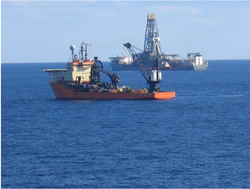
Figure 1.1: Dynamic positioning system: Offshore Support Vessel Toisa Perseus. In the background, the fifth-generation deepwater drillship Discoverer Enterprise can be seen. (Source: [Wikipedia, 2013])
