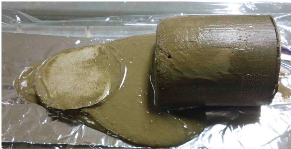
(a) Filter cake build-up after 30 s filtration time.
