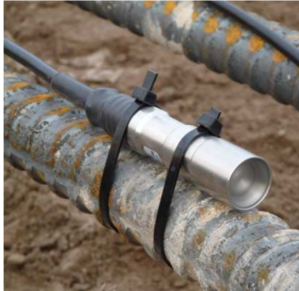
Figure 5.5: Pore pressure sensor used for measurements in Dörverden. The gel pad allows measurement of total stresses.
