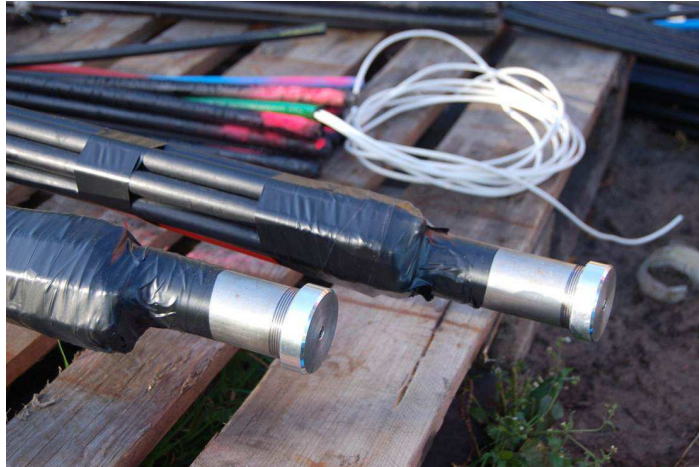
Figure 5.8: Casing for data logger and power supply attached to the tendon.
