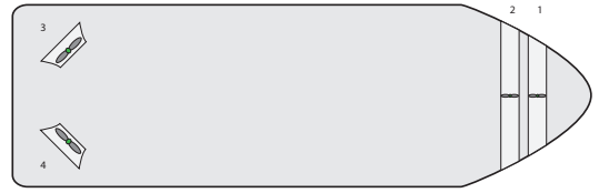
Fig. 2. The thruster layout of the simulated vessel.
