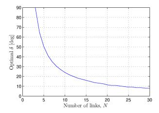
Fig. 6. The optimal phase shift  $\delta$  that maximizes the forward velocity of a planar snake robot as a function of the number of links N.
