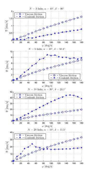
Fig. 8. The average forward velocity of the snake robot for different values of  $\omega$ . The number of links N and the corresponding values of  $\alpha$  and  $\delta$  are shown at the top of each plot.
