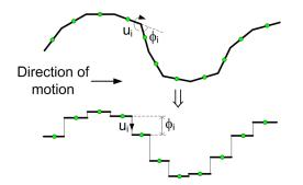
Fig. 3. The revolute joints of the snake robot are modelled as prismatic joints that displace the CM of each link transversal to the direction of motion.
