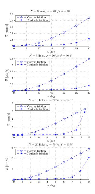
Fig. 7. The average forward velocity of the snake robot for different values of  $\alpha$ . The number of links N and the corresponding values of  $\omega$  and  $\delta$  are shown at the top of each plot.
