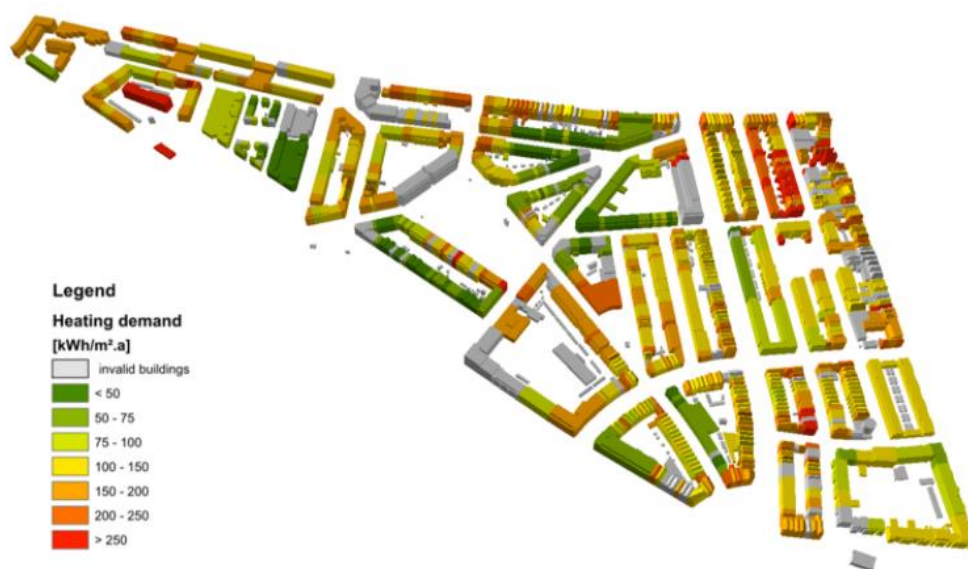
Figure 4 Overview of the heating demand for a large-scale energy project similar to Ludwigsburg (hft-stuttgart, 2018) .
