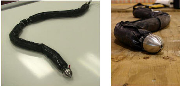
Figure 8: A snake robot with a skin drive propulsion system developed at Carnegie Mellon University. A motor drives the outer skin backwards along the snake body in order to propel the robot forward. Courtesy of Carnegie Mellon University.
