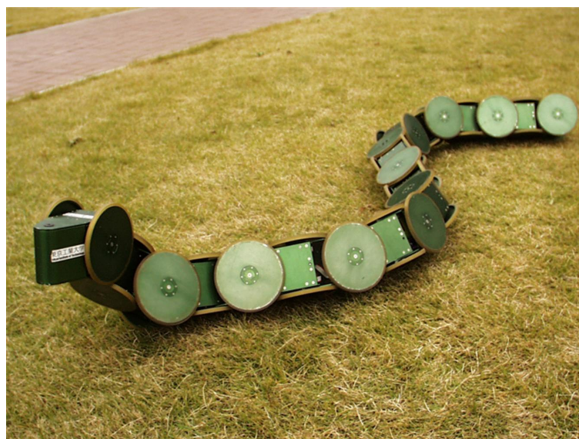
Figure 2: The snake robot ACM R3 developed at Tokyo Institute of Technology. The robot is covered with passive wheels. Courtesy of Tokyo Institute of Technology.
