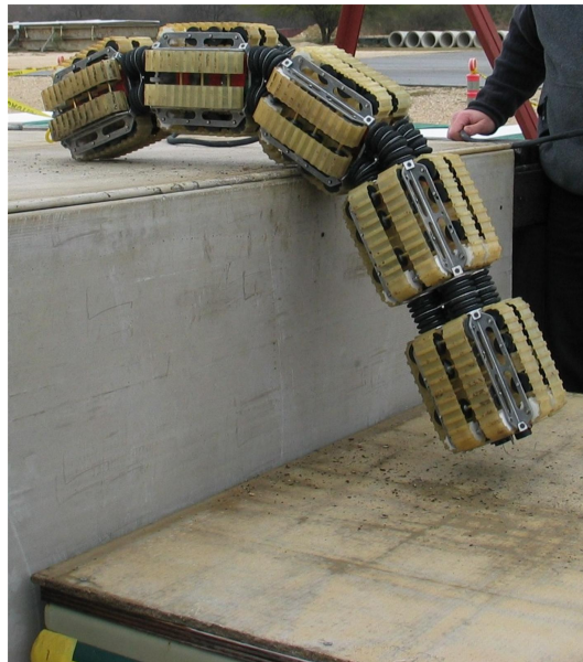
Figure 7: The OmniTread snake robot developed at the University of Michigan. The robot has pneumatic joints and is covered by motorized tracks. Courtesy of the University of Michigan.
