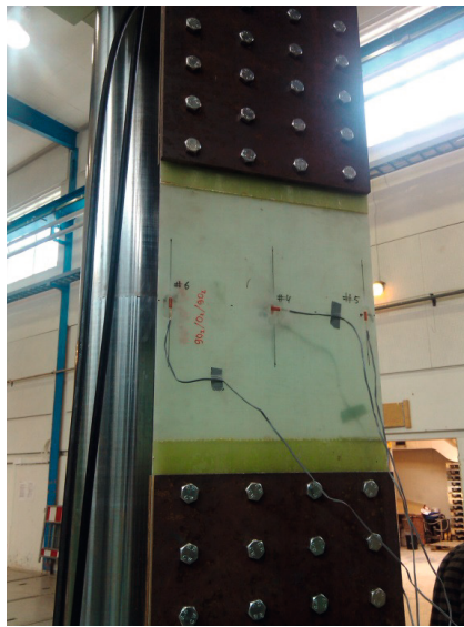
Figure 5.5. Specimen TR11\_1F in the 1000 kN test machine during fatigue loading.
