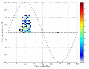
Figure 8. Discharge density plot versus phase angle of the AC voltage. Measured at 10 kV DC + 500  $V_{rms}$  AC, color bar shows number of discharges occurring during 20 minutes of applied voltage.
