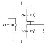
Figure 2. ABC equivalent circuit with RC-elements
