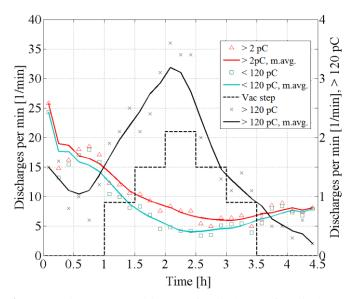
**Figure 7.** Discharge repetition rate for discharges for all, above and below 120 pC. 10 kV DC and 300, 500 and 700 V<sub>rms</sub>, at 80 °C. Sampling interval is 10 min. The y-axis on the left give the repetition rate for discharges above 120 pC.
