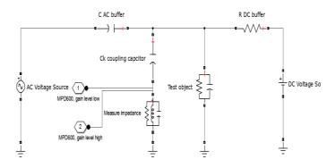
Figure 5. The test circuit – straight circuit with coupling capacitor.
