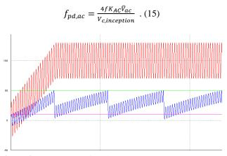
**Figure 3.** Breakdown of cavity voltage under combined AC and DC voltage, generalized plot. AC frequency lowered to better show the waveform. Red line: voltage over the test
