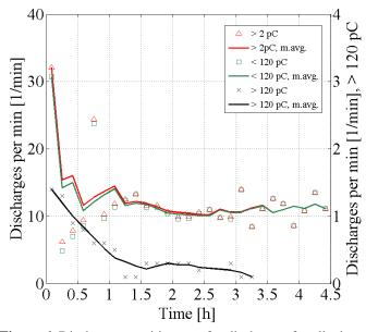
**Figure 6.** Discharge repetition rate for discharges for all, above and below 120 pC in test object at 10 kV DC, 80 °C. Sampling interval is 10 min. The y-axis on the left give the repetition rate for discharges above 120 pC.
